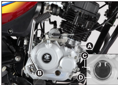
A : Oil Filler Cap B : Oil Level Gauge
